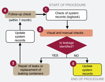
Steps 1 to 2 must be carried out always. If no leak is identified, the procedure is completed by updating the system records (logbook) (step 5).
